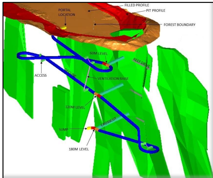
Kubi JV – oblique view looking SW to backfilled pit; showing proposed portal and decline, level crosscuts and reef drives, mineralization (after MBC, Ghana)
