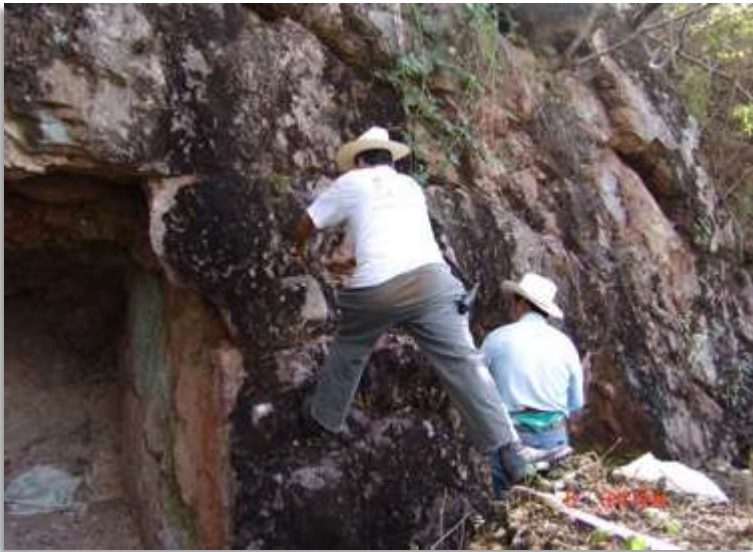
Fig. 8.27 Photo of Mina San Antonio. Sample 19856 cut from the pillar left below the samplers yielded results of 44.09 g/t Au, 47 g/t Ag, 0.4% Cu, 0.2% Pb, 0.7% Zn and 6.7% Fe. 图8.27为Mina San Antonio的图片，从采样人员左下方的柱子上切割下来的样品19856分析结果显示，黄金品位44.09克/吨、白银47克/吨、铜0.4%、铅0.2%、锌0.7%、铁6.7%。
