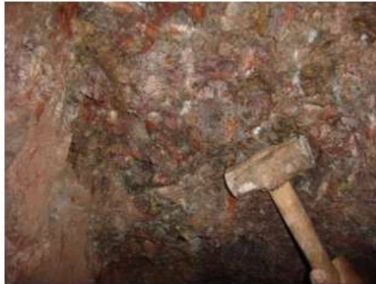
Fig. 8.21 Drift about 7 meters below and a few meters southwest from the point in Fig. 8.19 along the San Agustin Vein. Sample 105021 yielded a result of 148.2 g/t Ag and 60 g/t Au across 0.8 m.
