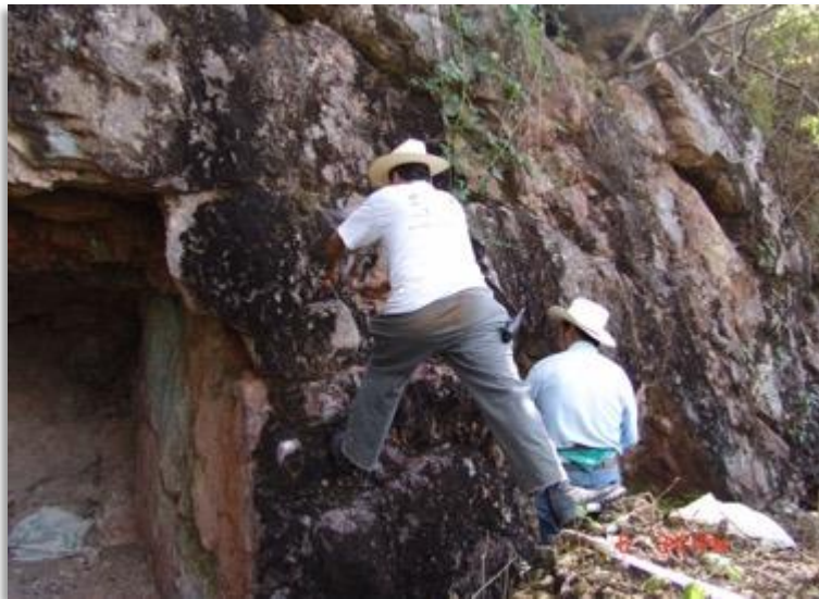
Fig. 8.27 Photo of Mina San Antonio. Sample 19856 cut from the pillar left below the samplers yielded results of 44.09 g/t Au, 47 g/t Ag, 0.4% Cu, 0.2% Pb, 0.7% Zn and 6.7% Fe.
