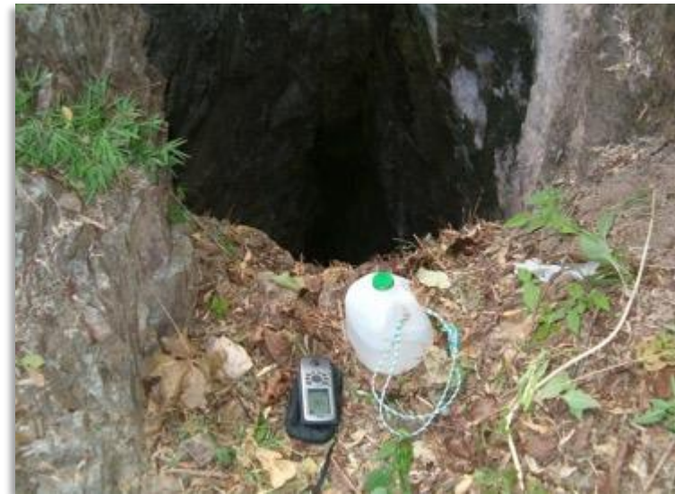
Fig. 8.26. Photo of Guayabo. A chip-channel sample across the vein yielded results of 5.2% Cu, 347 g/t Ag and 0.1 g/t Au across 0.7m (sample 15953).
