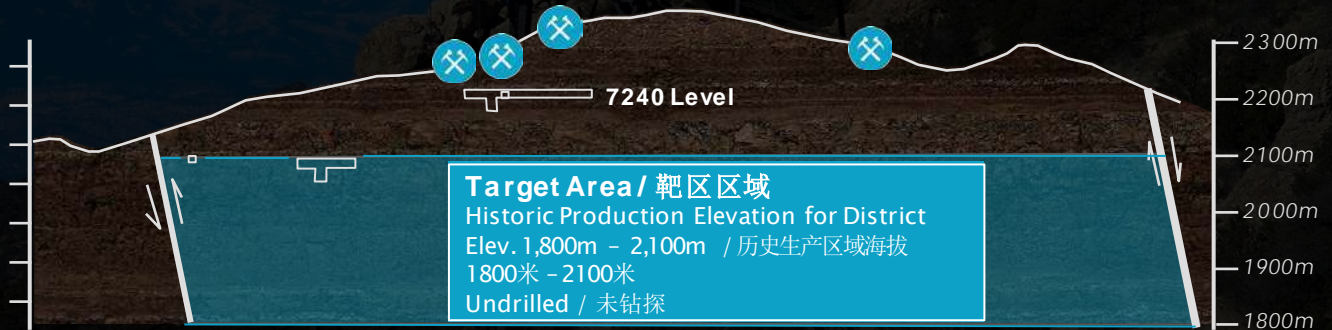
Simplified Longitudinal Section / 简化纵 向剖面图
