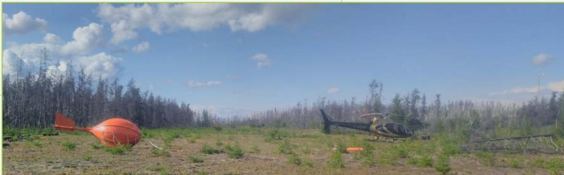
Airborne MT Survey at Shadow Project / Shadow项目的航空MT勘测
