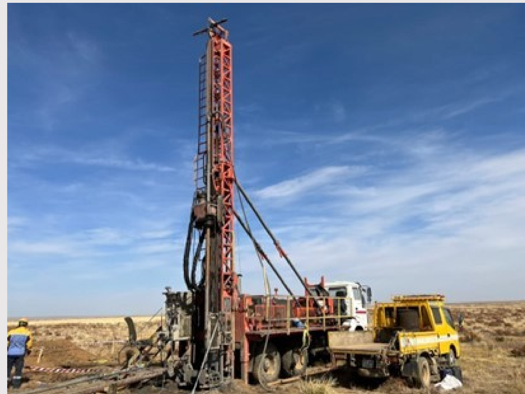
Diamond core drilling at UNDH-02 / 在UNDH-02的金刚石岩芯钻探
